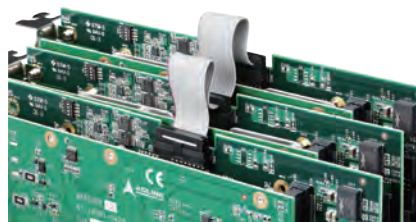
SSI bus cable for multiple card synchronization (For PCIe-9852)
